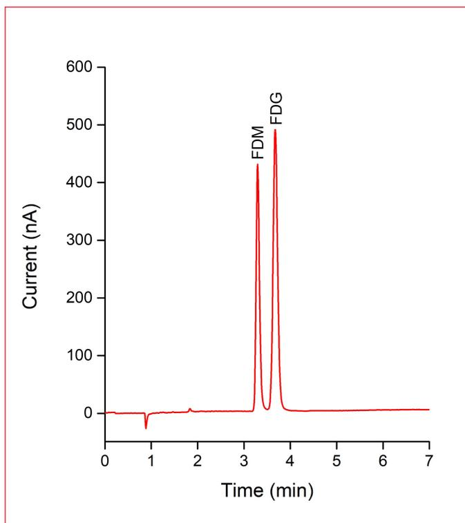
**Figure 3.** Chromatogram obtained with a 2 µL injection of the system suitability solution (reference solution c) consisting of 25 µg/mL FDM and 12.5 µg/mL FDG\* in DI water. FDG concentration in reference solution c based on a maximum recommended dose V of 20 mL.
