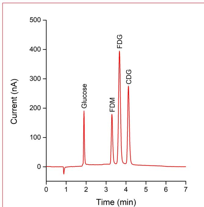
**Figure 2.** Chromatogram obtained from a standard mix consisting of 10 µg/mL FDG, FDM, CDG and 1 µg/mL glucose in DI water (2 µL injection). Resolution between FDM-FDG and FDG-CDG are 2.4 and 2.5, respectively.
